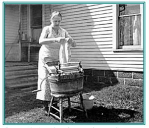
Figure 42 Manual washing machine with wringer
